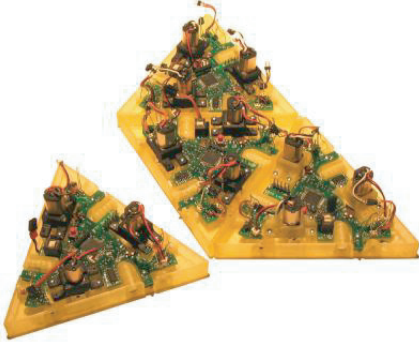
Fig. 1. Robotic “programmable parts” [4]. Each edge of a part may attach via a magnetic latch to another part. Once attached, the parts may communicate and decide to remain attached or may dis-attach by rotating a permanent magnet, which disengages the latch.
